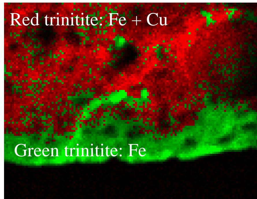
Micro x-ray fluorescence image –green coating at the top of red trinitite
